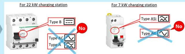
EV Renault Car Sharing project must respect all EV standards, especially charge infrastructure. Below the most important requirements, all driven by ZE Ready 1.4D compliance for hardware, installer and installation.
