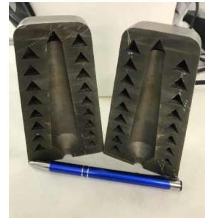
Cup Mold with Conformal Cooling Channels
