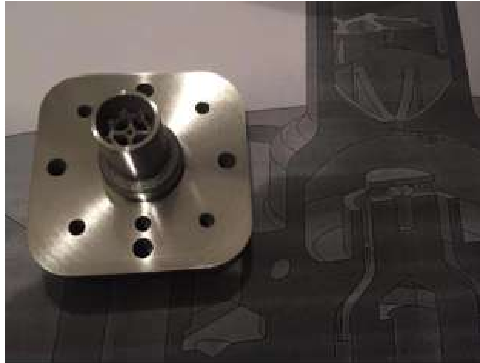
Combustor for SpaceX- Inconel 718
